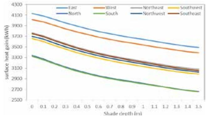
Fig. 11. Annual window heat gain for different orientations with variable shading depth
