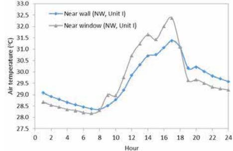
Fig. 5. Air temperatures near window and wall with same orientation.
