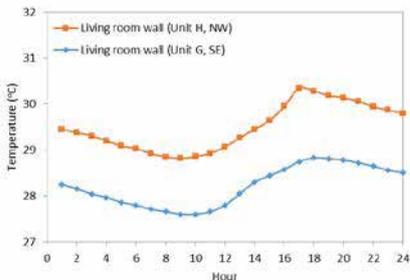
Fig. 4. Internal surface temperatures of walls with different orientations.
