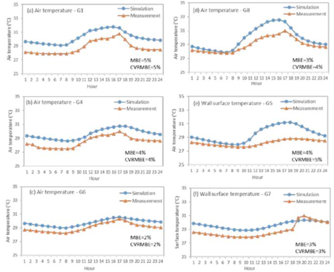
Fig. 8. Comparison between simulated and measured temperatures.
