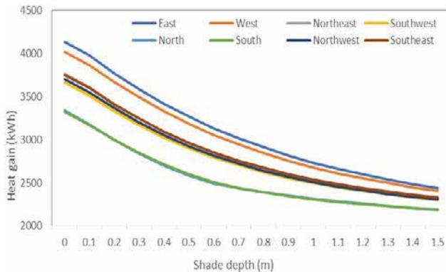
Fig. 10. Annual window heat gain with different depth of horizontal shading device
