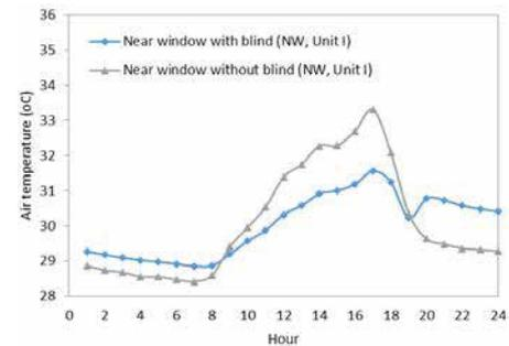
Fig. 6. Air temperature in common bedrooms with and without blind.
