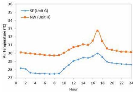
Fig. 3. Air temperature near walls with different orientations.
