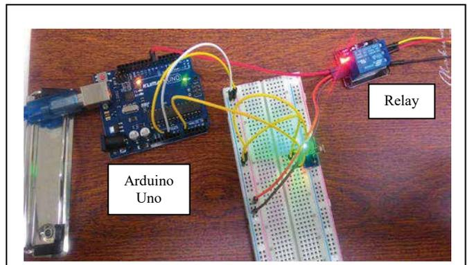
Fig. 5. Standard serial communication between relay and slave arduino
