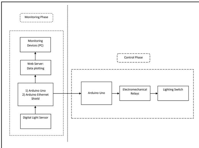
Fig. 2. Theoretical framework IoT platform for monitoring and controlling light intensity level
