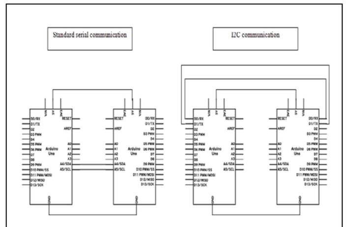
Fig. 4. serial communication for master and slave arduino
