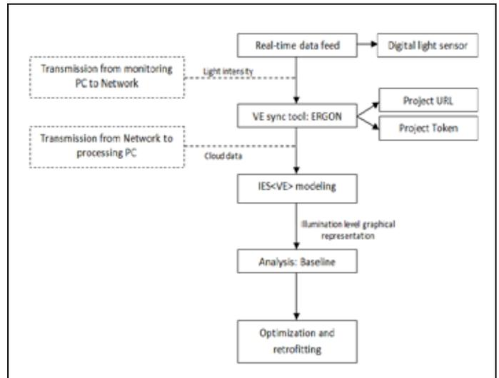
Fig. 1. IES-Ergon real time monitoring platform and common workflow. [9]
