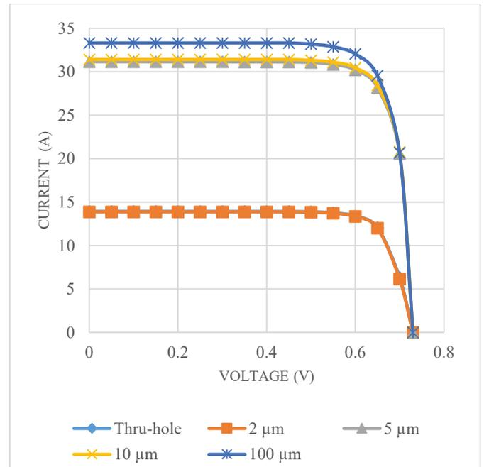
Fig 3: Simulated I-V curves for bifacial solar cell on partially transparent with different thickness of Si thin film for the transparency (100  $\mu\text{m}$ , 10  $\mu\text{m}$ , 5  $\mu\text{m}$ , 2  $\mu\text{m}$  and through-hole, 0  $\mu\text{m}$ ).
