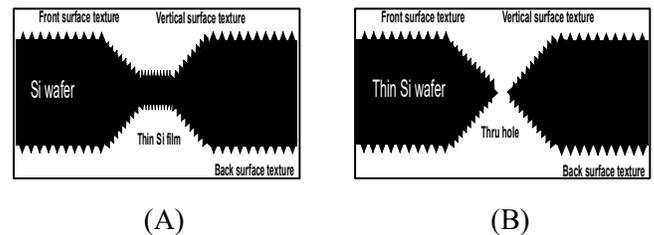
Fig 1: Pulsed laser processing conducted producing thin film (A) which allow light transmission to rear surface, and in the extreme case, though hole can be produce through high ns-regime or etching by using alkaline solution on laser area. Through hole allow 100% light transmission.
