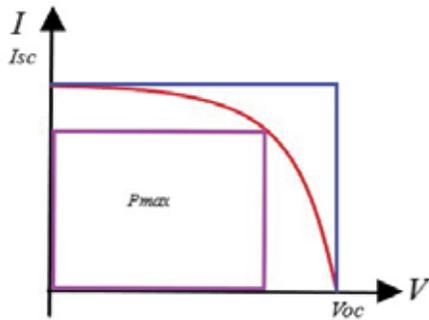
Fig 2: Maximum power rectangle ( $P_{max}$ ) is shows in  $I$ - $V$  curve for solar cell[17].
