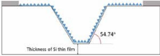
Fig 3: The pyramid structure is formed on wafer surface and trench slope at 54.74° with a variation of Si thin film thickness after drilling.
