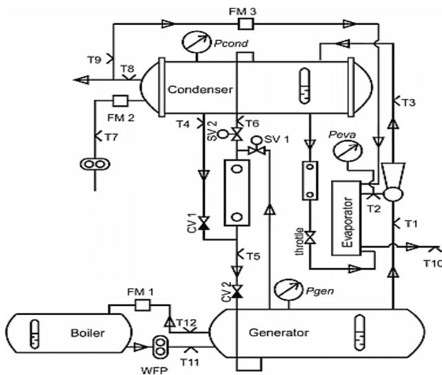
Fig 4. The experimental unit of ejector refrigerating system
