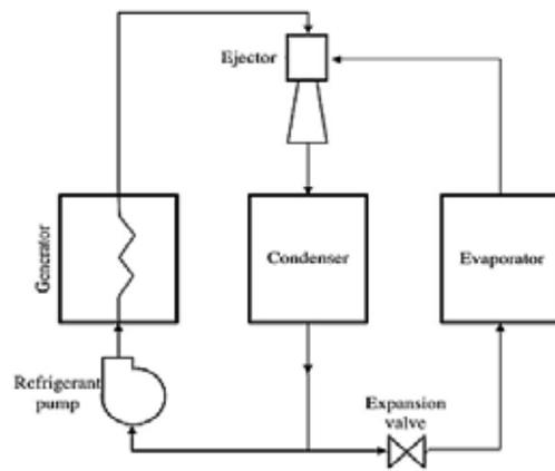
Fig 3. Cycle of ejector-based refrigeration system
