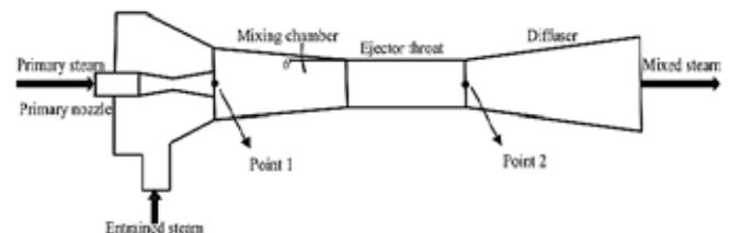
Fig 5. Parts of a typical ejector geometry
