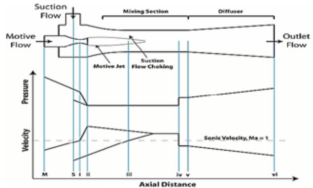
Fig 1. The operation of ejector system
