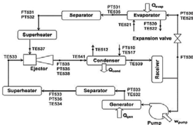
Fig 2 Ejector refrigeration cycle [1]
