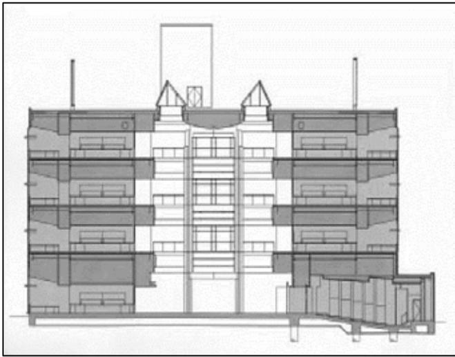
Fig. 4 shows the building section showing the interior atria, which provide daylighting (Source: Flad & Associates, Architect).
