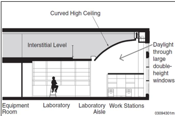
Fig. 2 shows the cross-section and photograph of the laboratory of Building 50 at the National Institutes of Health (NIH) complex (Source: U.S. Environmental Protection Agency [13])
