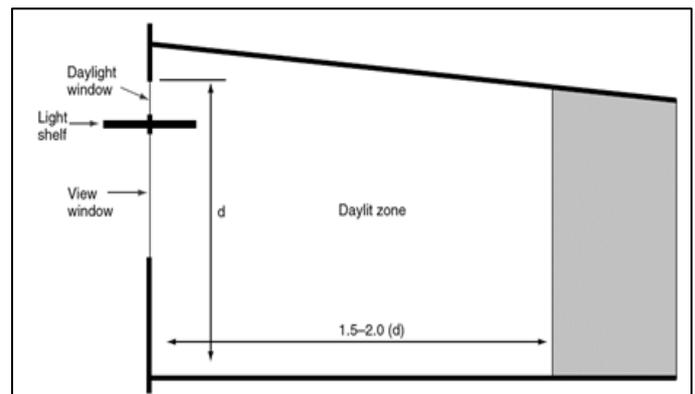
Fig. 1 shows a cross-section of a room to illustrate a rule of thumb for daylighting (Source: O'Connor et al. [11]).
