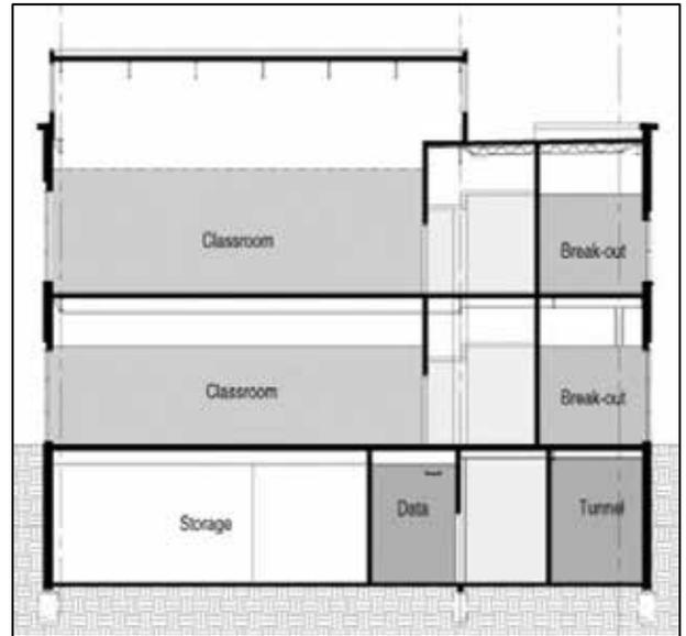
Fig. 3 shows the section through classroom block of the Centre for Technology and Learning Media building (Source: U.S. Environmental Protection Agency [13]).
