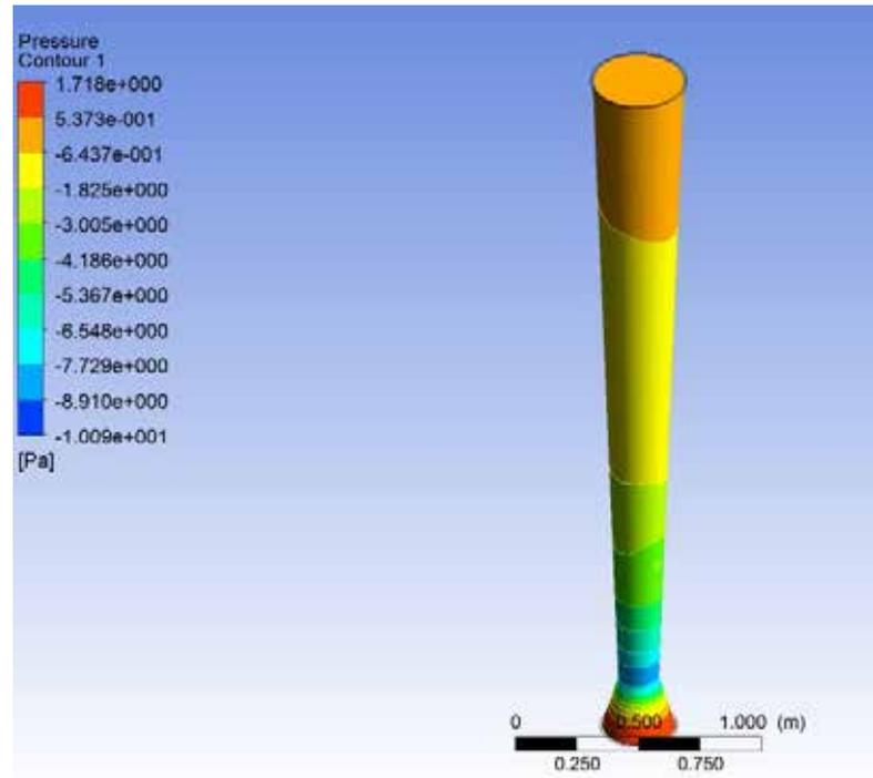
Figure 2: Pressure distribution inside the solar chimney
