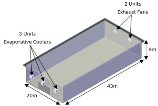
Fig. 1. Layout of warehouse with the evaporative coolers where the data logging exercise was conducted
