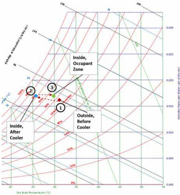
Fig. 9. Process of evaporative cooling for 11:00 on a psychrometric chart
