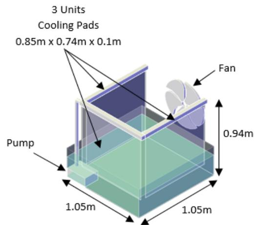
Fig. 3. Diagram showing the dimensions of the evaporative cooler installed at the warehouse
