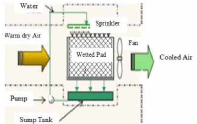
Fig. 2. Schematic diagram of direct evaporative cooler [8]
