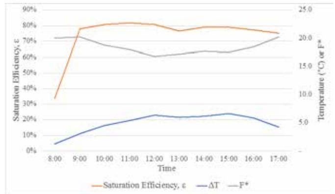
Fig. 6. Average hourly saturation efficiency curve for the evaporative cooler,  $\Delta T$  and  $F^*$
