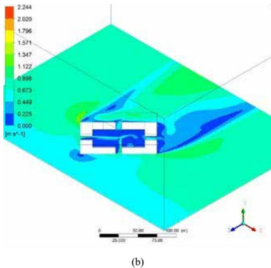
Fig. 4. 45° wind angle, (a) atrium with two access corridors, (b) atrium with four access corridors
