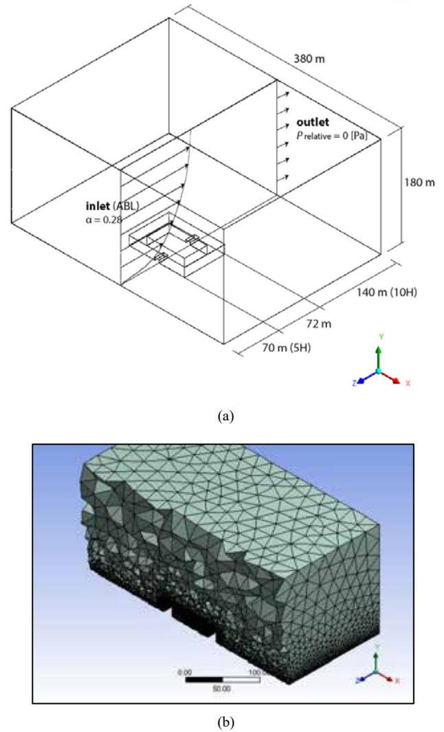
Fig. 1. (a) The boundary condition set up for the simulation, and (b) the tetrahedron meshes
