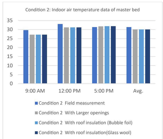
Fig.9.Changes in indoor air temperature in different simulations (Condition 2)
