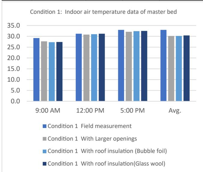
Fig.8.Changes in indoor air temperature of master bed in different simulations (Condition 1)
