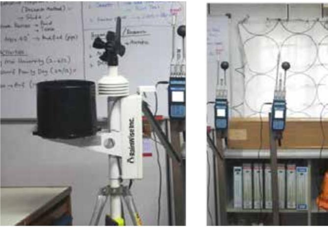
Fig. 3. Calibration of all instruments in the indoor control environment
