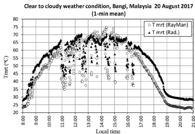
Fig. 2.  $T_{mrt}$  as calculated by six directional radiation method and the simulated  $T_{mrt}$  by RayMan1.2 software.
