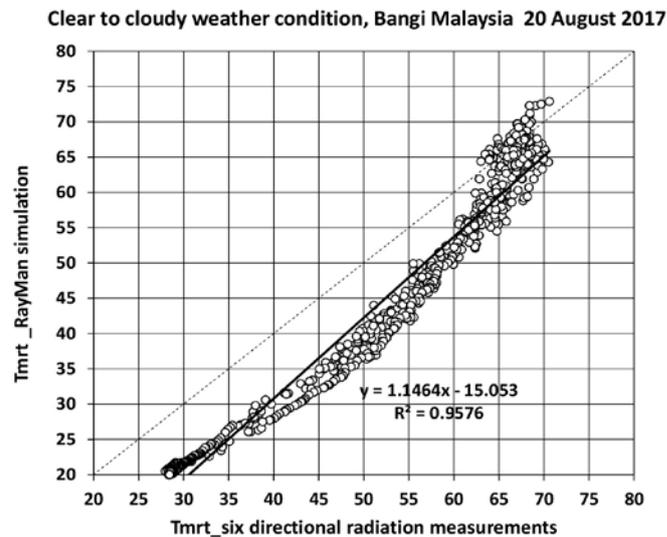
Fig. 3.  $T_{mrt}$  as calculated by six directional radiation measurements vs. simulated by RayMan 1.2 software.
