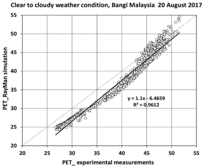
Fig. 4. PET as calculated by experimental measurements vs. simulated by RayMan 1.2 software.
