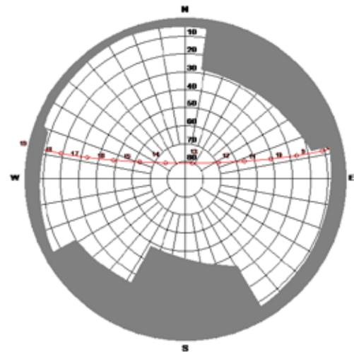
Fig. 1. An illustration of the fish-eye view and sun duration at the measuring site as simulated by RayMan
