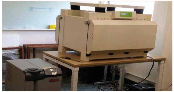
Fig. 1. Heat flow meter FOX600 model
