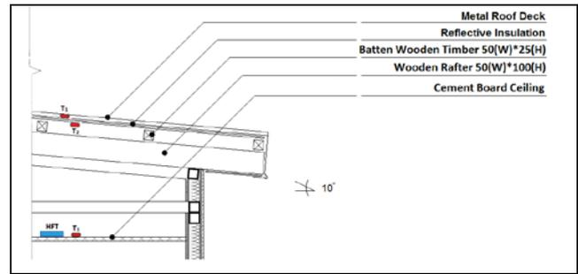
Fig. 5: Locations of Thermocouples for Phases 6-7 (Dimensions in mm)
