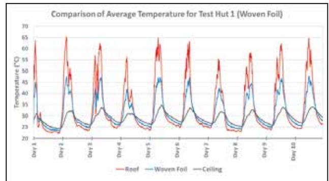
Fig 6: Average temperature for roof tiles, woven foil and ceiling
