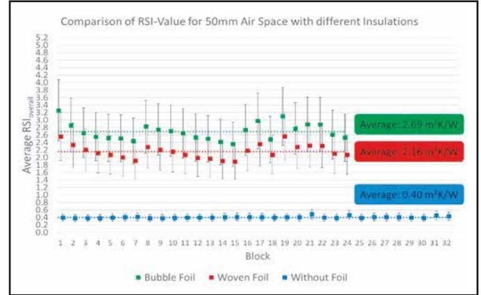
Fig. 8: RSI results for 3 test huts
