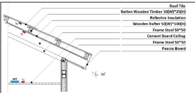
Fig. 4: Locations of Thermocouples for Phases 1-5 (Dimensions in mm)
