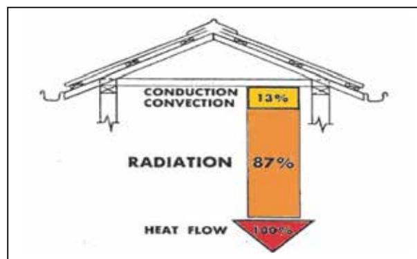
Fig 1: Heat Flow Mechanisms
