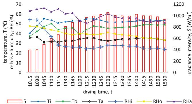
Fig. 3: Value for irradiance intensity  $S$ , temperature  $T$  and relative humidity  $RH$  of drying chamber and ambient data.
