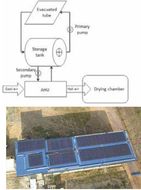
Fig. 1: System diagram (top) and top view of evacuated tube (bottom)
