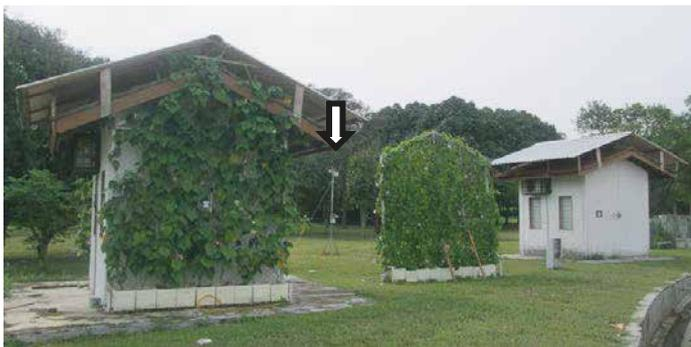
Fig. 1. Experiment setup of test cells; control test cell (right) and green façade test cell (left) and weather station (white arrow).
