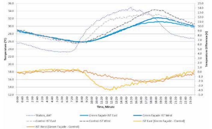
Fig. 3. Internal surface temperature (IST) for control and green facade walls for eastern and western orientations. Temperature difference shown the cooling effect performance of the green facade.
