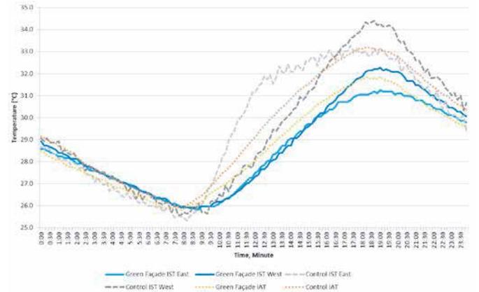
Fig. 4. Thermal performance of internal surface temperature (IST) and indoor air temperature (IAT).
