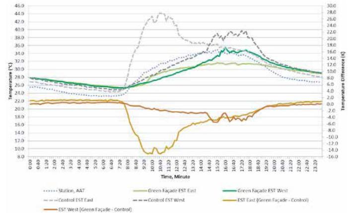
Fig. 2. External surface temperature (EST) for control and green facade walls for eastern and western orientations. Temperature difference shown the cooling effect performance of the green facade.
