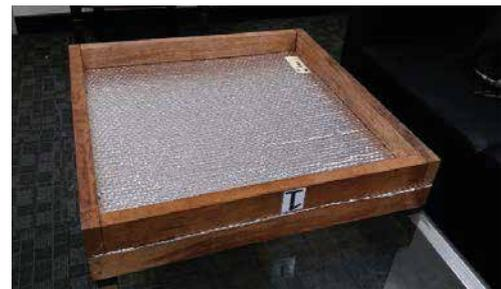
Fig. 4. Timber frames are used to create top and bottom air gaps for bubble foil for heat flow measurement
