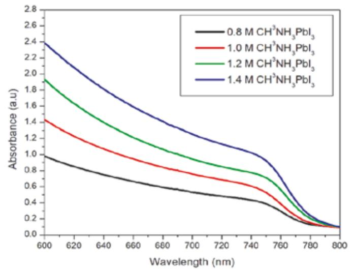
Fig. 3. UV-Vis absorbance spectra of 0.8 M, 1.0 M, 1.2 M and 1.4 M  $\text{CH}_3\text{NH}_3\text{PbI}_3$  films.
