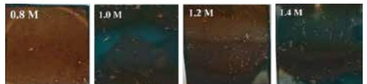
Fig. 4. The TiO<sub>2</sub>/CH<sub>3</sub>NH<sub>3</sub>PbI<sub>3</sub> films on FTO glass with 0.8 M, 1.0 M, 1.2 M and 1.4 M CH<sub>3</sub>NH<sub>3</sub>PbI<sub>3</sub> precursor concentrations.
