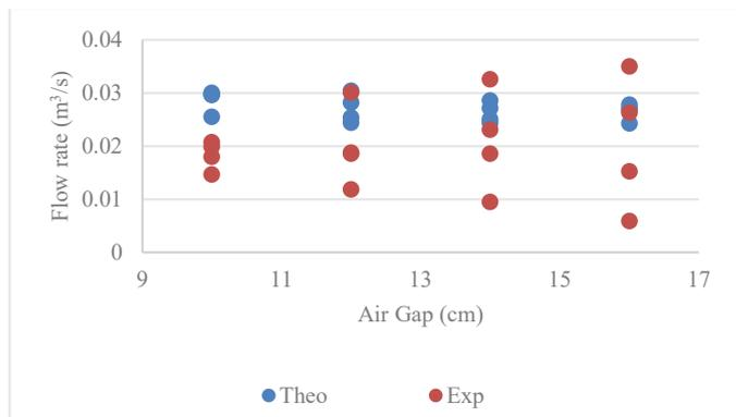
FIGURE 4: COMPARISON BETWEEN EXPERIMENTAL VALUES WITH THEORETICAL VALUE FOR DIFFERENT AIR GAP
