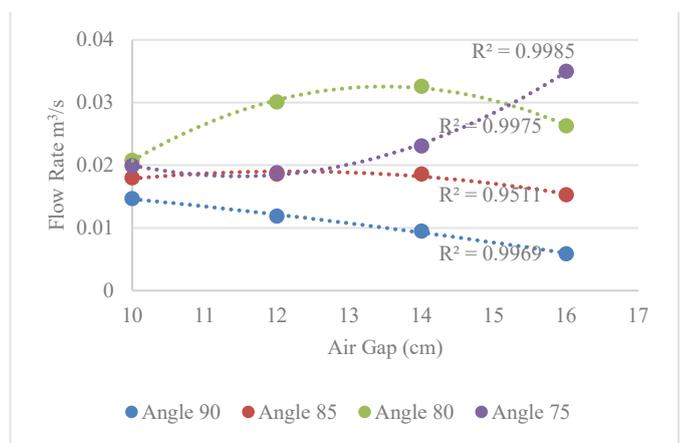
FIGURE 2: RELATION BETWEEN AIR FLOW RATE AND AIR GAP FOR DIFFERENT CHIMNEY MODEL
