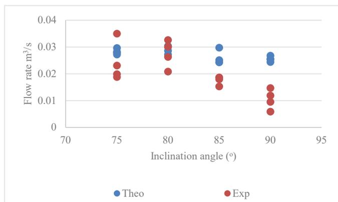
FIGURE 5: COMPARISON BETWEEN EXPERIMENTAL VALUES WITH THEORETICAL VALUE FOR DIFFERENT INCLINATION.
