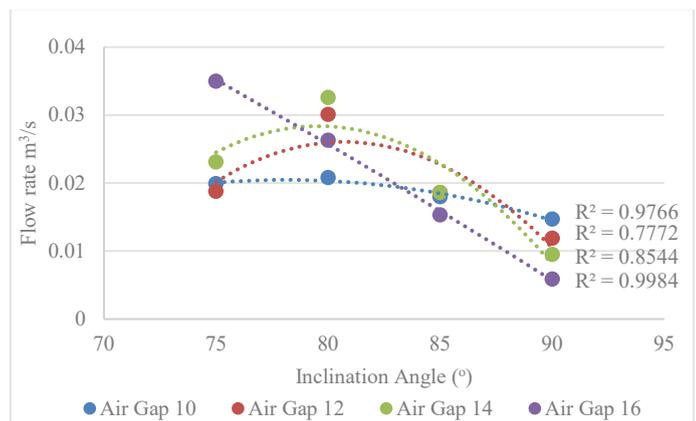
FIGURE 3: RELATION BETWEEN AIR FLOW RATE AND
