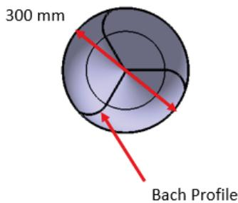
Fig. 5. The Savonius Bach profile and the diameter of the Savonius blades.
