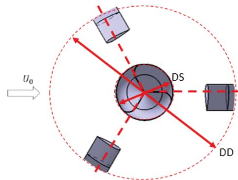
Fig. 4. Attachment angle between Darrieus blades and Savonius blades (dotted lines) and diameter of both Darrieus and Savonius blades (DD and DS),  $U_0$  is the depiction of wind direction example.
