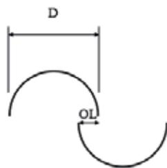
Fig. 6. Overlap between two Savonius blades.
