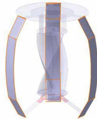
Fig. 3. Darrieus blades of the wind turbine (highlighted).
