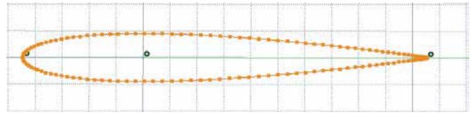
Fig. 2. NACA 0012 airfoil profile selected for Darrieus blades.
