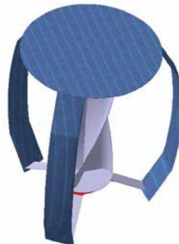
Fig. 10. 3D model rendering of solar thin film integrated to the Darrieus blades and to the thin circular plate on top of the wind turbine.
