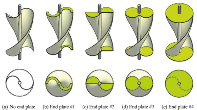
Fig. 8. Configurations of end plates tested on the Savonius blades. [9]
