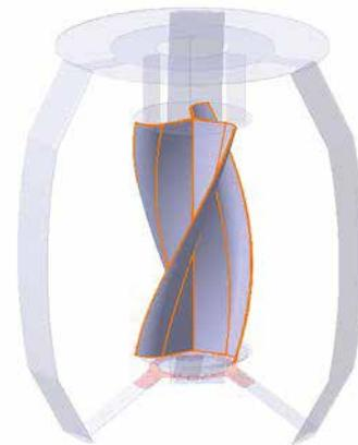
Fig. 7. Savonius blades of the wind turbine (highlighted).
