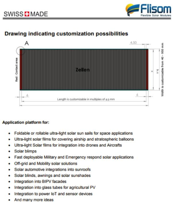
Fig. 9. Screen grab from Flisom product brochure, depicting the flexible thin film, as an example film suitable for this turbine.
