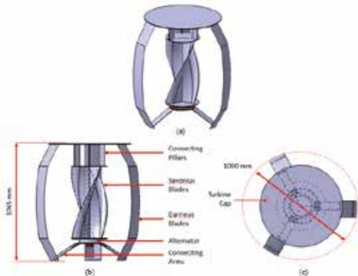
Fig. 1. Isometric view of the solar-integrated hybrid wind turbine (a), and its general parts from side view (b) and top view (c).
