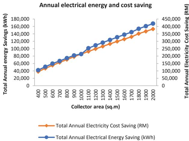
Fig. 5 Total annual electrical energy and cost saving to existing hot water plant
