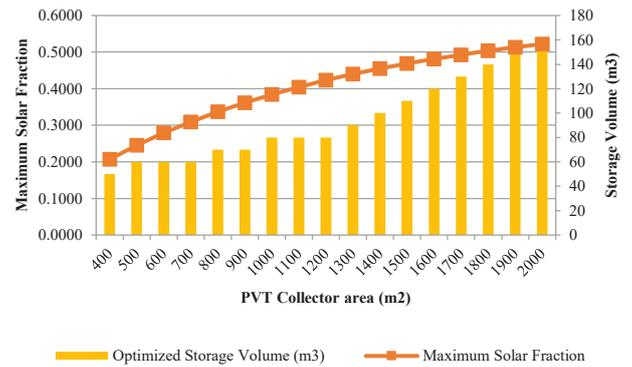
Fig. 3 Effect of storage volume on solar fraction with different PVT collector area
