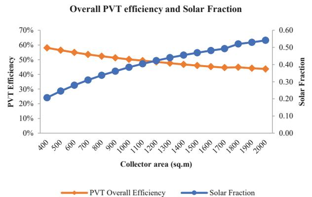
Fig. 4 PVT efficiency and solar fraction for different PVT collector area
