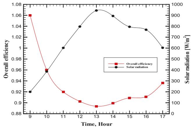
Figure 6. Variation of overall efficiency of PV/T evaporator Overall efficiency was reported to be higher in the mornings and afternoons due to the influence of the (higher) ambient temperature, while efficiency was reported to be lowest during noon, which is attributed to the high solar radiation increasing the surface temperature of the PV. When the surface temperature of the evaporator decreases to levels under the ambient temperature, the evaporator collect heat not only from
