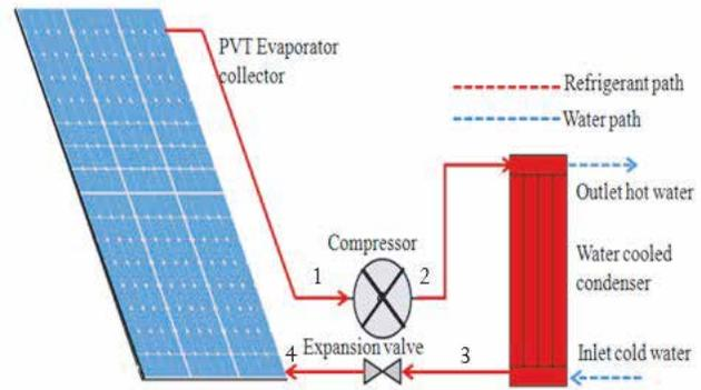
Fig. 1: Schematic diagram of PV/T-Heat Pump system direct-expansion (DX-SAHP) and Water heating system.
