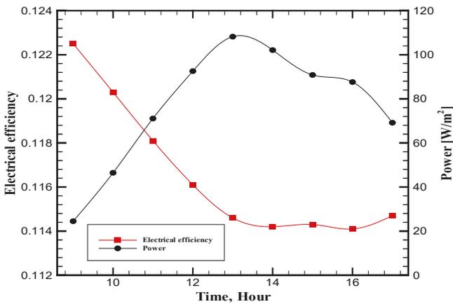
Fig. 4 Variation of electrical efficiency and PV power output
