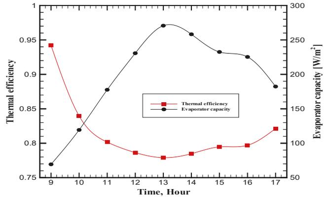
Fig.5 Variation of thermal efficiency and evaporator capacity
