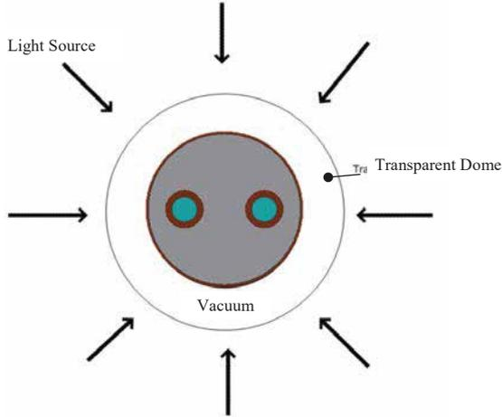
Figure 2.1: Physical Configuration of Solar Thermal Energy Storage using PCM Tube
