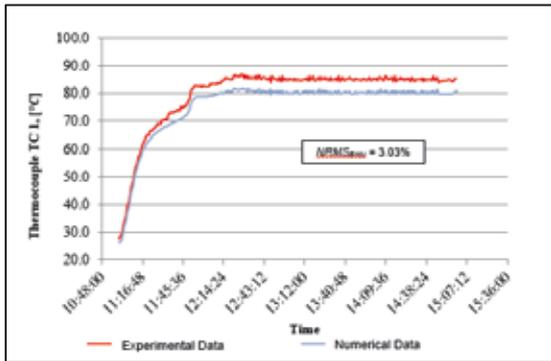
Figure 3.3: Experimental and Numerical Comparison of Thermocouple TC 1 Temperature Results. (Mass flow rate of  $2.217 \times 10^{-4}$  kg/s)
