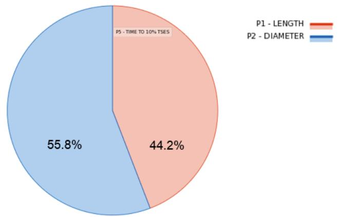
Figure 4.7: Sensitivity of Each Design Parameter toward Time Required to Reach 10% of Total Specific Energy Storage.
