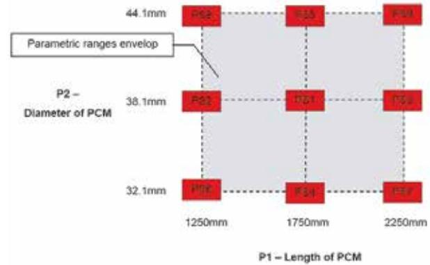
Figure 4.1: Design Points generated from CCD Design Method.
