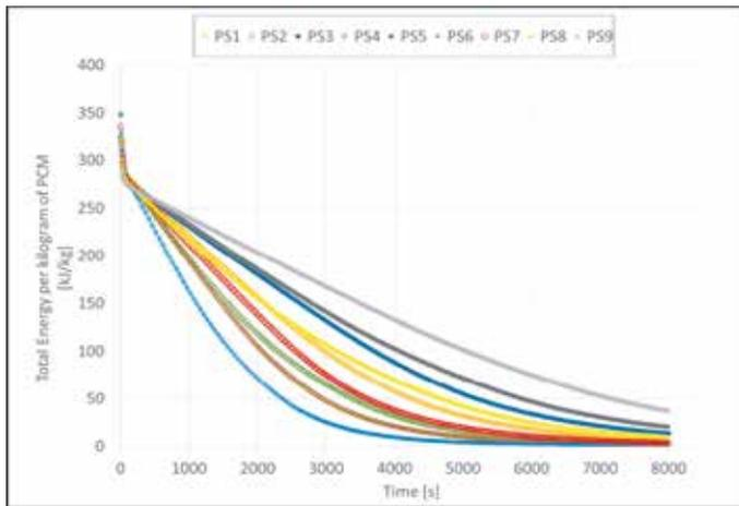
Figure 4.6: Total Specific Energy Storage Comparison for Different Design Points.
