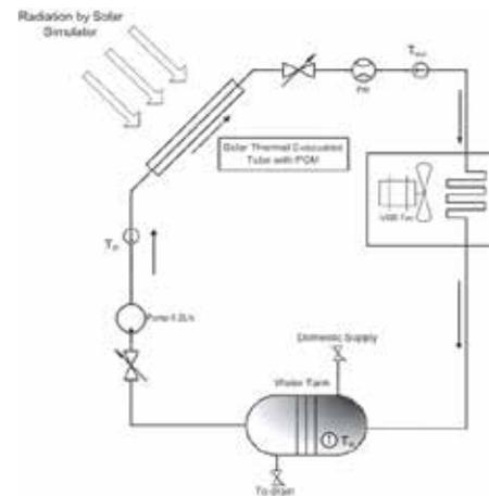
Figure 3.1: Experimental Solar Thermal Evacuated Tube with PCM Schematic Diagram.
