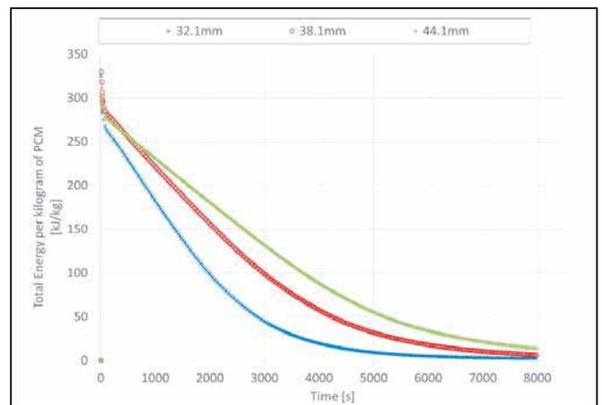
Figure 4.5: Total Specific Energy Storage Comparison for Different Tube Diameter.
