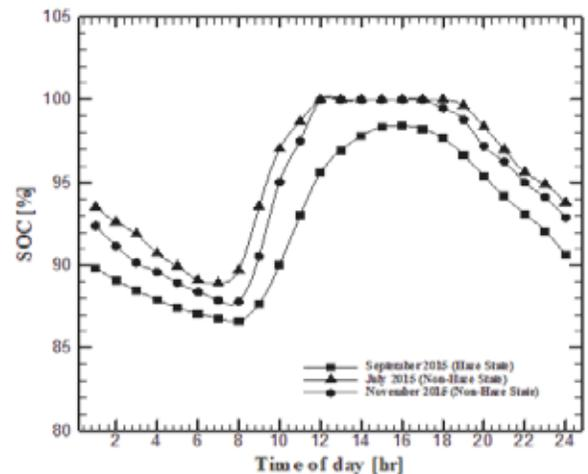
Figure 5. The Monthly Average of State of Charge (SOC %) for the batteries in the months; July 2015 (Non-Haze State), November 2015 (Non-Haze State) September 2015(Haze State)
