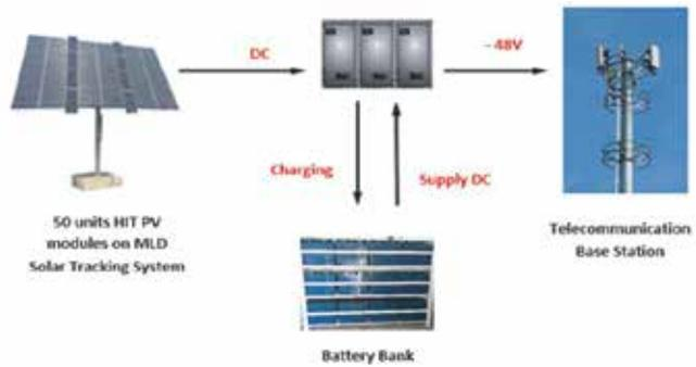
Figure 3. Block diagram of Double Axis HIT modules with MLD
