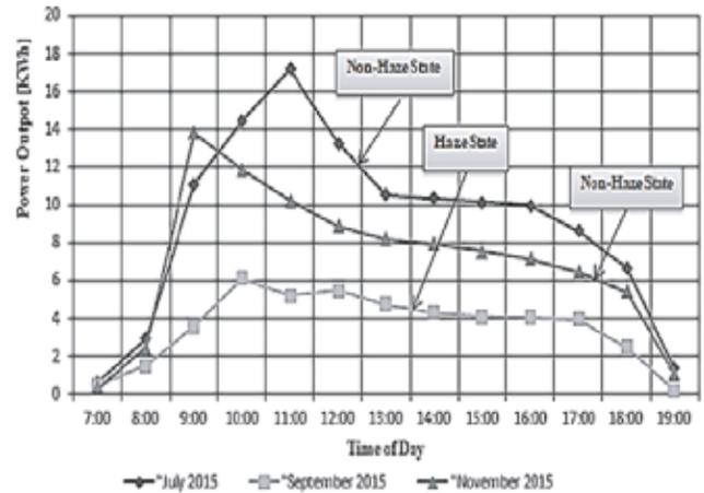
Figure 4. Power output from MLD dual axis PV module.
