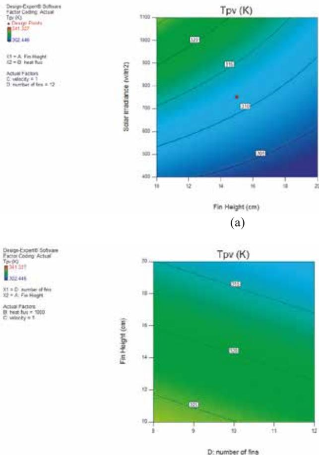
Fig 5 (a) effect of solar irradiance and truncated fin height (b) effect of truncated fin height and number of fins on the mean PV module temperature reduction
