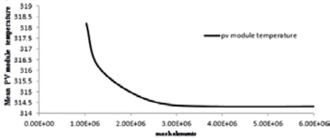
Fig.2 Mean PV module temperature over mesh face for GIT
