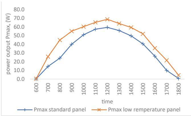
Fig. 9: Value of  $P_{max}$  for standard and low temperature panel.
