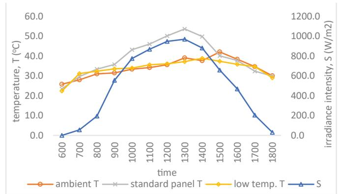
Fig. 7: The values of  $S$ , ambient  $T$ , standard panel  $T$  and low temperature panel  $T$ .
