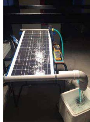
Fig 3: Low temperature panel tested indoor under solar simulator.
