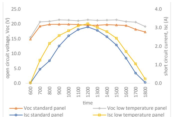
Fig. 8: The  $V_{oc}$  and  $I_{sc}$  values for first comparison.
