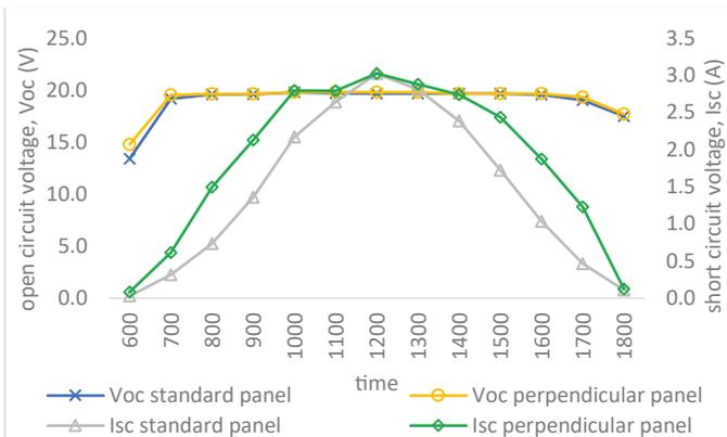
Fig 10: The  $V_{oc}$  and  $I_{sc}$  for second comparison.
