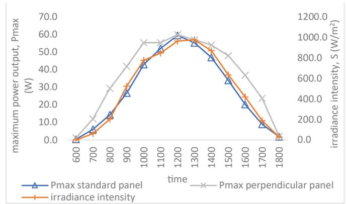
Fig 11: The  $S$  and  $P_{max}$  values for standard and perpendicular panel.
