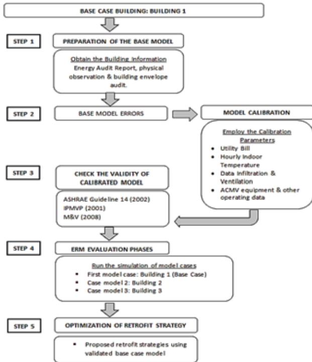
Fig. 4. Five steps in developing model cases and retrofit strategies using a calibrated simulation approach.
