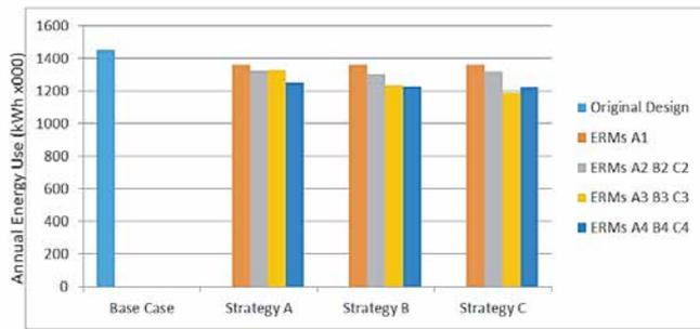
Fig. 9. Comparison for space cooling energy consumption reduction of retrofit strategies.
