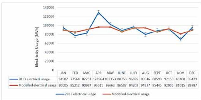
Fig. 5. Monthly comparison of 2013 case model electrical usage (utility bills) with simulated model of monthly electrical usage.
