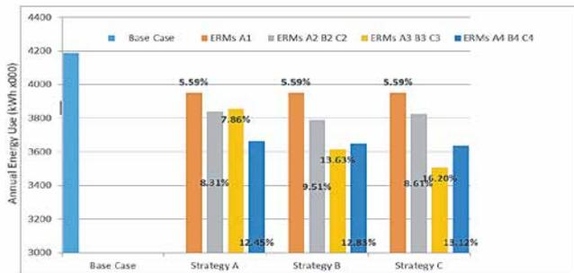
Fig. 10. Comparison for annual energy consumption of ERMs with base case.
