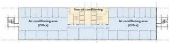
Fig. 1. Typical upper floor plan of Buildings 1 and 2 with two different thermal zones.
