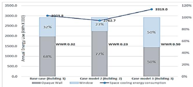
Fig. 7. Comparison of modelled annual energy consumption by opaque and window components for all simulated case models.
