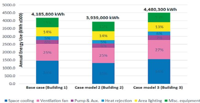
Fig. 6. Comparison of modelled annual energy consumption by end use components for all simulated case models.
