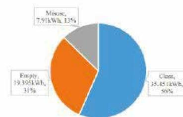
Fig. 4. The total lighting electricity usage of 12 lecture rooms in two-week monitoring period.
