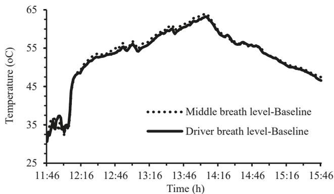
Fig. 6. Comparison between middle and driver breath level air temperatures, Day 1.
