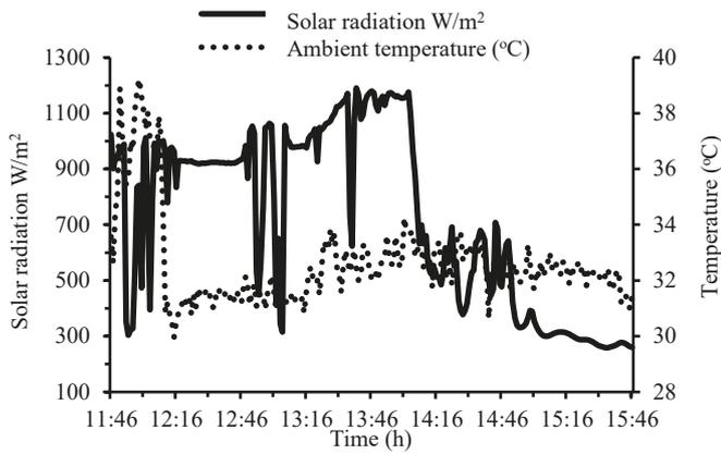
Fig. 5. Solar irradiance and ambient air temperature measurements, Day 1
