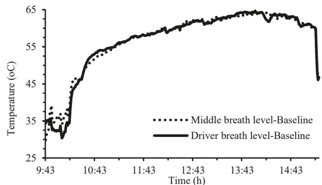
Fig. 8. Comparison between middle and driver breath level air temperatures, Day 2
