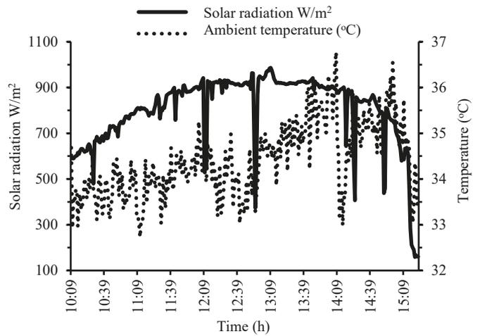
Fig. 7. Solar irradiance and ambient air temperature measurements, Day 2
