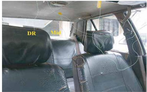
Fig. 4. Thermocouples located at breath-level of driver (DR) & middle cabin location (Mid)
