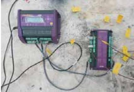
Fig. 2. Datataker DT80 during field measurements
