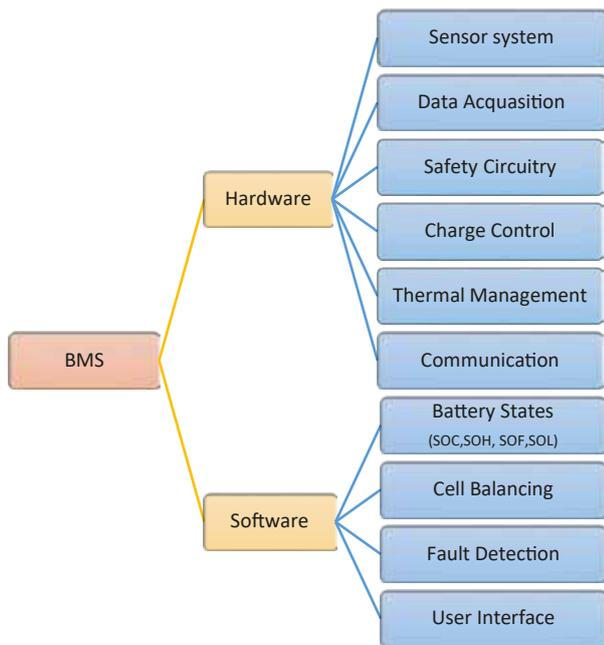
Fig. 2. Basic component of BMS in EVs
