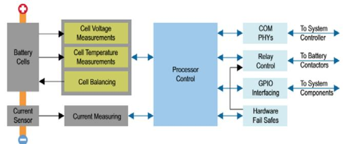
Fig. 3. Block diagram of BMS[19]
