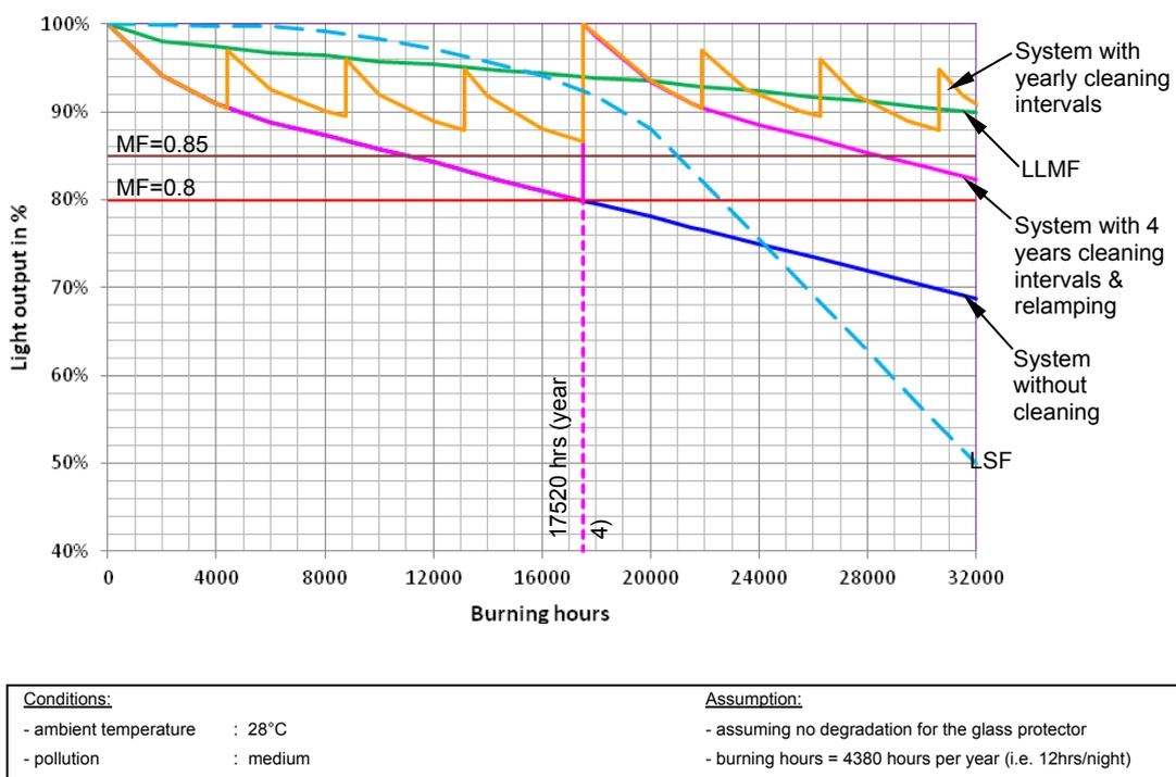
vi) From Figure 4, in order to ensure that the safe lighting level is maintained the cleaning interval for LED luminaire shortens progressively with operating hours thus presenting additional challenges in maintenance and budget planning.
