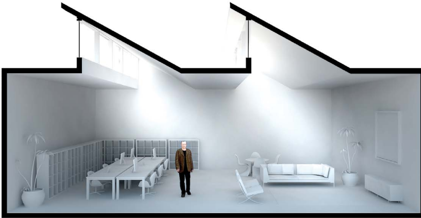
FIGURE 4.6.2 | TYPICAL SAW-TOOTH ROOF LIGHT DAYLIGHT HARVESTING
