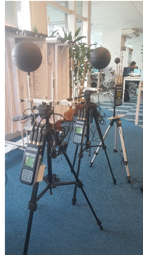
Images: IEQ measuring devices setup at Lendlease Office in Menara Binjai
